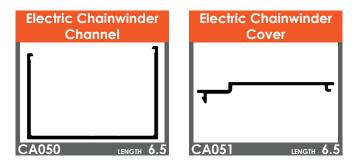
The **Electric Chainwinder Chainnel** is designed to suit the high quality Assa Abloy Elevation Electric chainwinder. This device is compatible with standard Cbus and BMS systems, but can also be controlled from an optional Assa Abloy touch screen display or even rain sensors.
