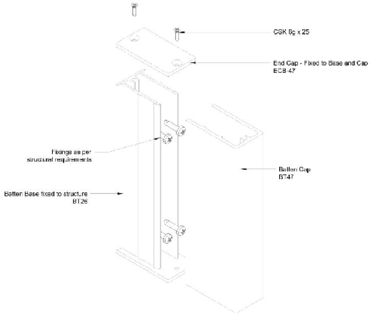
The 25mm Batten System includes the following three profiles.
