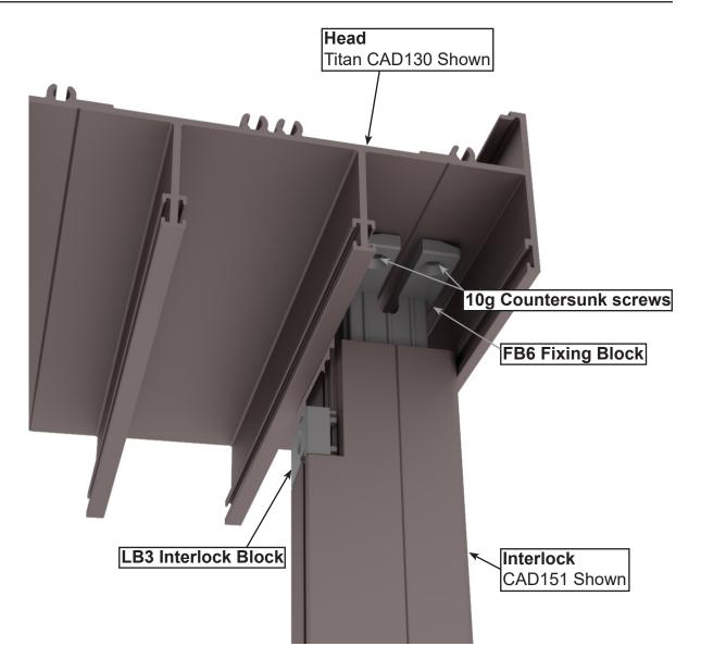
The FB6 is designed to have a tight fit. It is possible to have a small amount of variance in the alumnium extrusions that will result in the FB6 being too tight. In this case, it is recommended to lightly shear one side of the block to help fitment.
