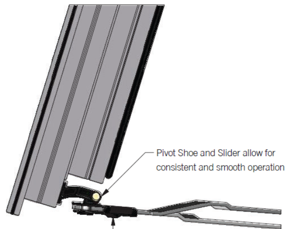
Heavy Duty Four-bar Stainless Steel Stays provide balancing action for smooth operation
