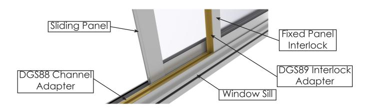
The **DGS89** is riveted directly to the back of the fixed panel interlock. It includes an overlapping leg that covers the side of the flyscreen, and allows an **FC1** clip to be used to hold it in place.
